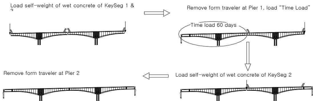
**Consideration of age difference using Time Load for Construction Stage Analysis**
