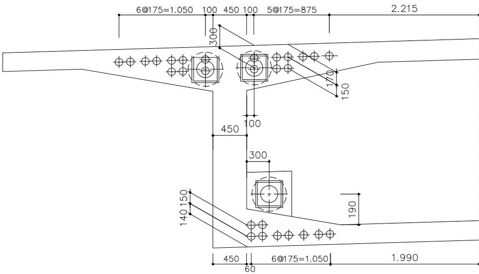
**Tendon Arrangements for the Center Span**
