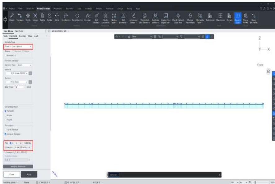
**Generation of left half of bridge using beam elements**
