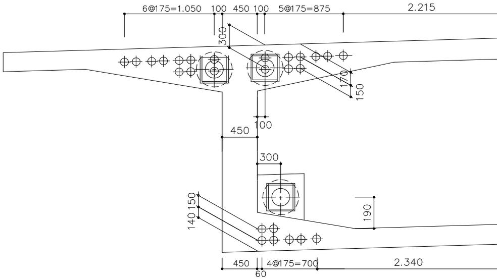
**Tendon Arrangements for the Side Span**
