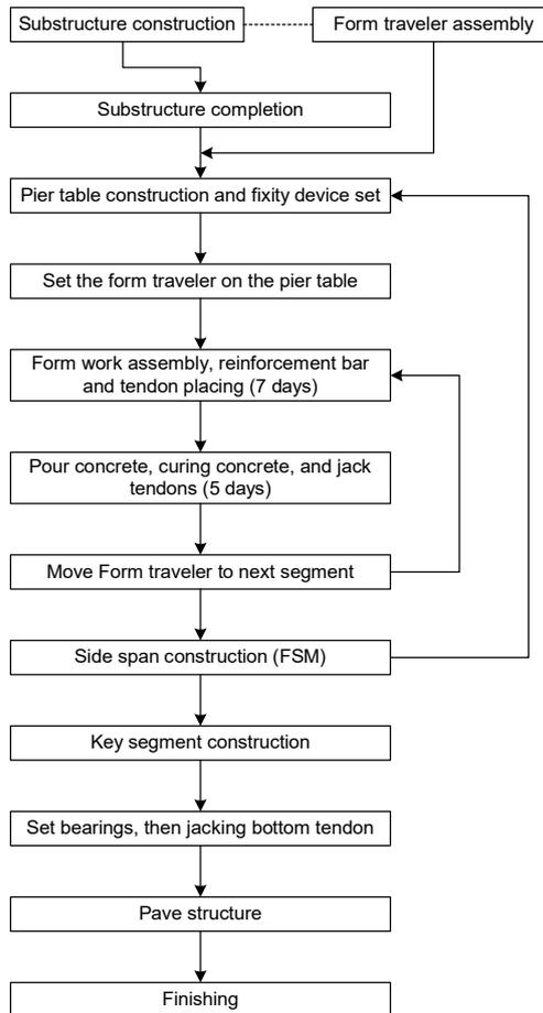
Note: This example is a 3-span FCM bridge constructed with 4 Form Travelers (FT).
